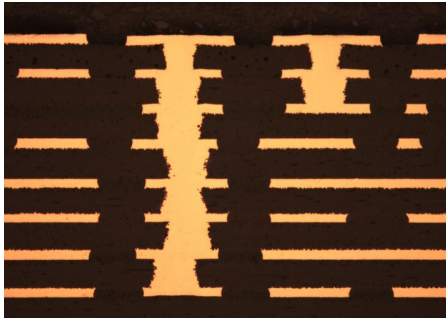
Stacked via with ELIC technology
